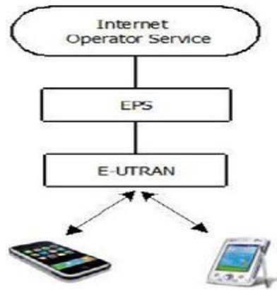
**Figure1 EPS (LTE/SAE) Architecture**
