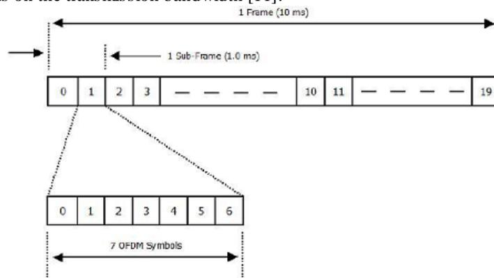
Figure 4 Frame Structure
