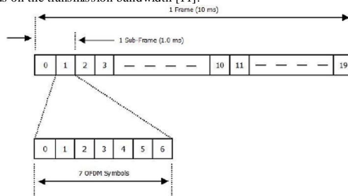
Figure 4 Frame Structure
